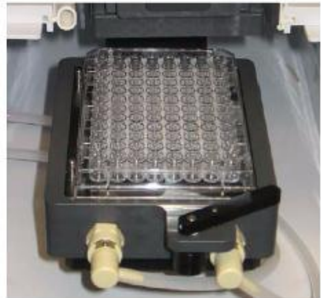
Plate loader on ACDC
